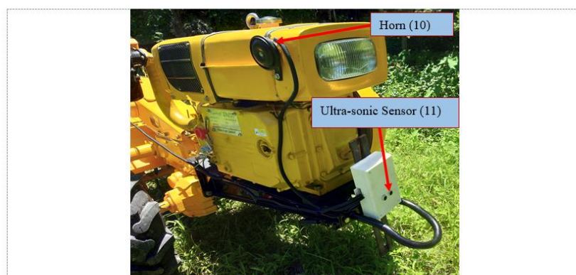
Fig. Automatic safety stop incorporation with remote controlled turning mechanism
